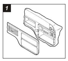
Disconnect the negative battery terminal to prevent an accidental short circuit. Unclip the right side of the dash trim bezel. Unclip the left side of the bezel and remove. Remove (3) 7mm hex-head screws securing the factory head unit and disconnect the wiring.
